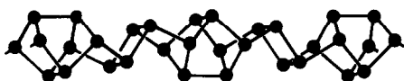
FIG. 3. A cutout of the tube-like chains of phosphorus atoms in the structure of \text{Cu}_2\text{P}_3\text{I}_2 . One translation period of the chain consists of 24 P atoms arranged in two \text{P}_8 units—with a structure like the molecular compound \text{As}_4\text{S}_4 (11)—which are bridged by squares of P atoms in two different orientations.
